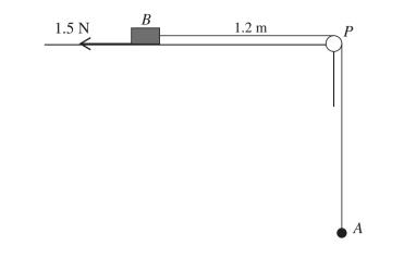
A particle A and a block B are attached to opposite ends of a light elastic string of natural length 2 m and modulus of elasticity 6 N. The block is at rest on a rough horizontal table. The string passes over a small smooth pulley P at the edge of the table, with the part BP of the string horizontal and of length 1.2 m. The frictional force acting on B is 1.5 N and the system is in equilibrium (see diagram). Find the distance PA. [3]
