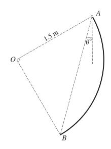
A uniform rigid wire AB is in the form of a circular arc of radius 1.5 m with centre O. The angle AOB is a right angle. The wire is in equilibrium, freely suspended from the end A. The chord AB makes an angle of  $\theta^{\circ}$  with the vertical (see diagram).
