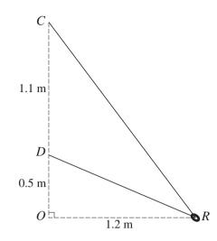
One end of a light inextensible string is attached to a point *C*. The other end is attached to a point *D*, which is 1.1 m vertically below *C*. A small smooth ring *R*, of mass 0.2 kg, is threaded on the string and moves with constant speed  $v \text{ m s}^{-1}$  in a horizontal circle, with centre at *O* and radius 1.2 m, where *O* is 0.5 m vertically below *D* (see diagram).
