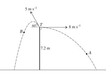
Particles *A* and *B* are projected simultaneously from the top *T* of a vertical tower, and move in the same vertical plane. *T* is 7.2 m above horizontal ground. *A* is projected horizontally with speed  $8 \text{ m s}^{-1}$  and *B* is projected at an angle of  $60^{\circ}$  above the horizontal with speed  $5 \text{ m s}^{-1}$ . *A* and *B* move away from each other (see diagram).
